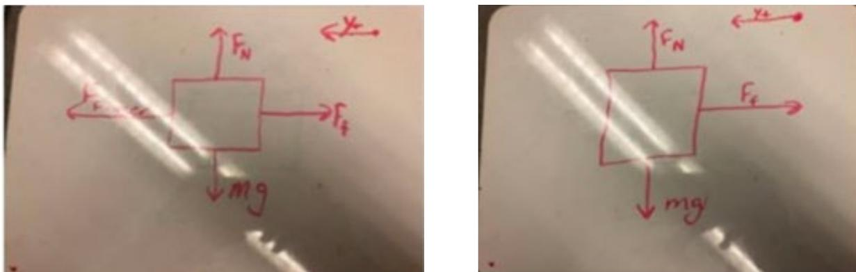
Figure 4: Force diagrams from the students' lab report, one including the force of the push (on the left, captioned "When pushing IOLab" by students) and one without (on the right, captioned "After we release the IOLab" by the students).
