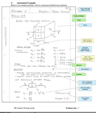
A substantial portion of any problem is understanding what the problem is (problem statement) and how to represent it in engineering terms (model). When making the model, such as converting a 2x4 stud wall into four elements of varying thermal conductivity, you are making and showing your engineering assumptions. Textbook problems often do this for you and show the model you should use directly, as in the following example.
